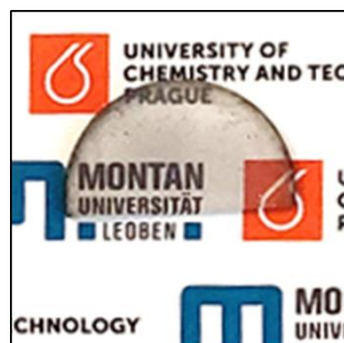
Fig. 1: Transparent alumina prepared by templated grain growth in SPS.
